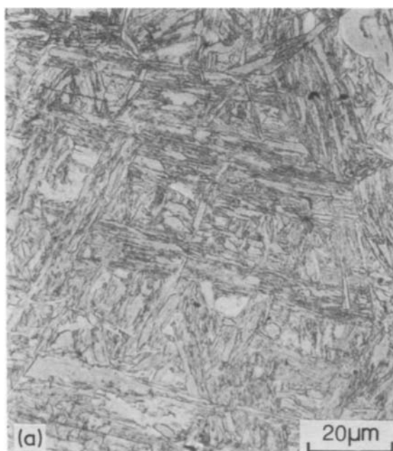
Figure 4 Optical micrographs obtained at various cooling rates: (a) 30\,000 , (b) 8400 , (c) 2700 , (d) 900 , (e) 140 , and (f) 55^{\circ}\text{C min}^{-1} ; PAGB = prior austenite grain boundary, A = an apparent sheaf, WF = Widmanstätten ferrite-like plates, PF = polygonal ferrite.
