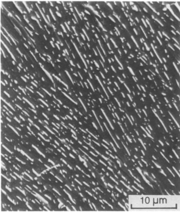
Figure 7 Scanning electron micrograph of the B_2 structure after deep etching.
