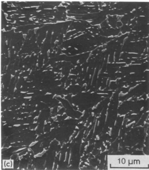
Figure 11 Scanning electron micrographs for the transformation products obtained at cooling rates of (a) 2300, (b) 1980 and (c) 1200 °C min -1 .
